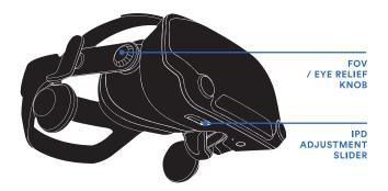
To optimize image clarity, move the IPD adjustment slider while wearing the headset. This moves the lenses to match the distance between your eyes.
