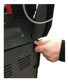
To access your keyboard and mouse, first unscrew the two thumb screws from the backplate.
