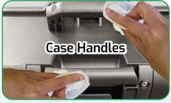
**Disinfectants with a high alcohol percent may damage your devices.** VRSim recommends Lysol or Clorox disinfectant wipes for effective cleaning. Do not use hand sanitizer on SimSpray.
